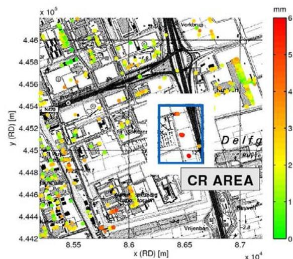
Figure 11. Visualization of the amplitude of the periodic signal, estimated through the joint estimation of the linear velocities and periodic signal.
