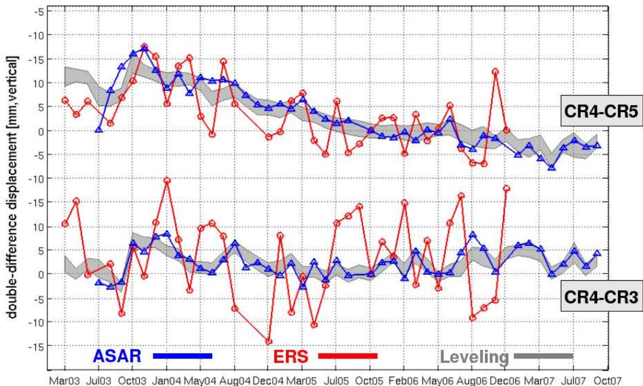
Figure 5. Time history of InSAR double differences, before sub-pixel correction, compared to leveling double differences. A gray stripe indicates a range of  $\pm 1.5$  mm of standard deviation of leveling measurements. The estimated standard deviation of double-difference InSAR phase in this case are 10.7mm (vertical) for ERS-2 while 2.4mm (vertical) for Envisat.
