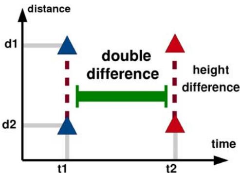
Figure 3. Leveling double-differences: “first in space then in time”.
