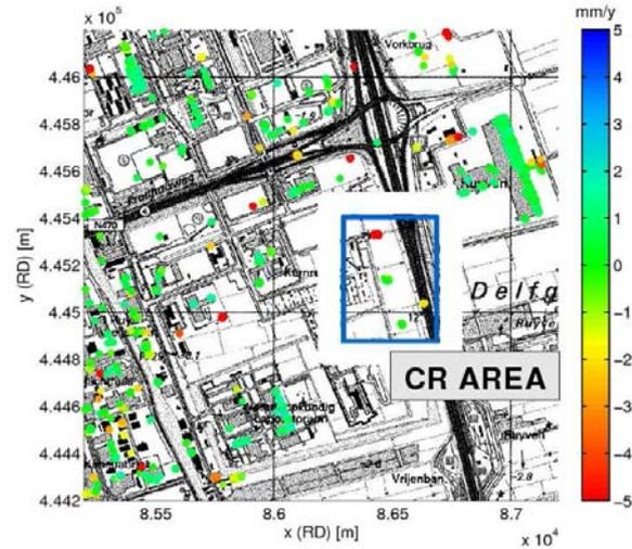
Figure 10. Linear velocities in the corner reflectors area. The standard Delft PSI processing chain was applied.
