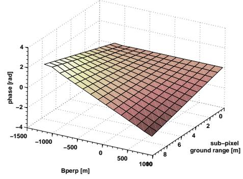
Figure 17. Systematic phase offset in the range direction as a function of scatterer location and perpendicular baseline.
