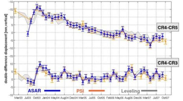
Figure 13. Time history of double differences of PSI, InSAR and leveling. Corner reflector 4 used as reference. The correlation coefficient between deformation estimates obtained by InSAR and PSI is on average higher than 95%. The error bars of InSAR double-difference empirically estimated, showing that all measurement techniques are in agreement within the error bounds.
