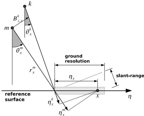
Figure 16. Geometry for a point target located at a sub-pixel position in range.
