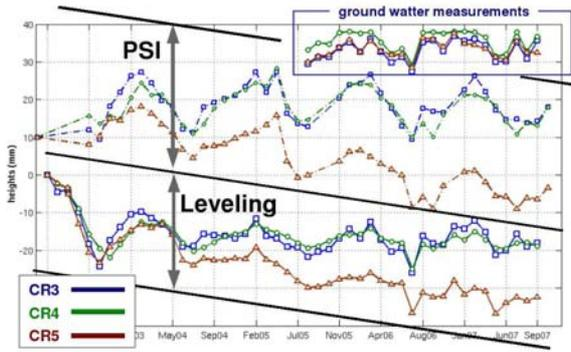
Figure 12. Comparison of time histories of PSI estimated (periodic) deformation and levelling. Note that PSI results are referenced to the arbitrary reference PS that is considered to be stable and not influenced by seasonal effects.
