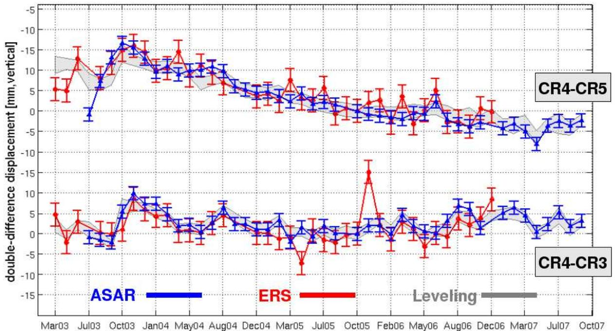
Figure 8. Visualization of empirically derived error bars of InSAR double-differences. The error bars represent the precision of each measurement technique between “ $1-\sigma$ ” criterion. The results show that the measurement techniques, i.e. leveling and InSAR, are in the agreement within the error bounds. This plot can be also considered as a conclusion of this study.
