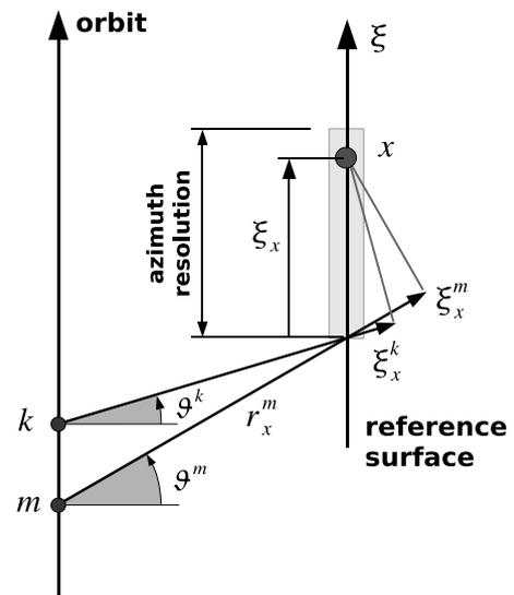
Figure 14. Geometry for a point target located at a sub-pixel position in azimuth.
