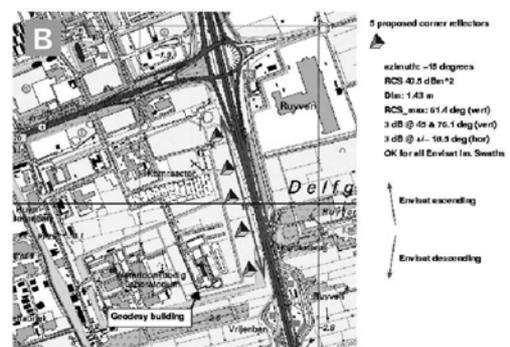
Figure 1. A topographic map of the corner reflector area and details of the radar cross section of the reflectors.
