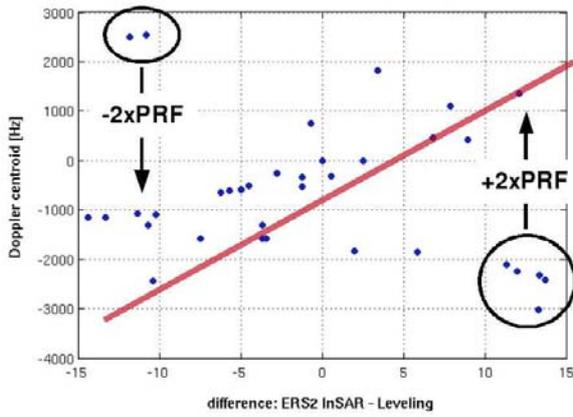
Figure 9. A scatter plot of ERS-2 InSAR – leveling differences as a function of Doppler centroid frequency of stacked ERS-2 images. The blue circles indicate an ambiguity in annotated Doppler centroid frequency values.
